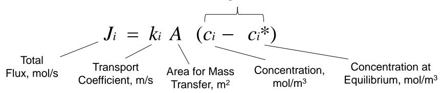
For J<sub>i</sub>>0 and finite k<sub>i</sub>, need infinite stages and infinite area
